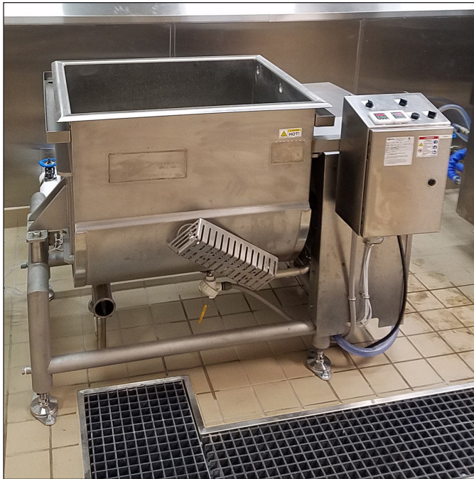
TECV-100S-P shown with optional 3" air-operated, flush-mounted drop-down valve
