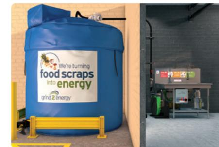
The energy rich slurry is stored on-site in a 3000-6000 gallon tank until hauler transports to AD facility.
